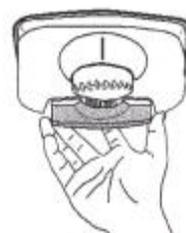
Replace the light cover by inserting the rear lug and pushing up to locate the two front lugs.
