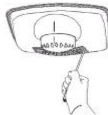
Use a flat tipped screwdriver to remove the light cover by inserting
