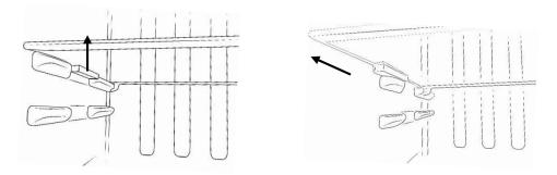
You can adjust the racks in the fridge and freezer compartments to your required configuration. To remove a rack hold both sides of the rack, lift it upwards (1) and then pull it towards you (2).
