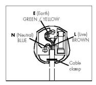
The wires in the mains lead are coloured in accordance with the following code: Green and Yellow = Earth Blue = Neutral Brown = Live
